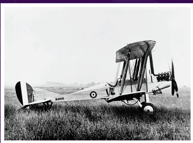
BE2c, two-seat reconnaissance aircraft, used by the Royal Flying Corps (RFC) during the First World War. Photo courtesy of Imperial War Museum.
