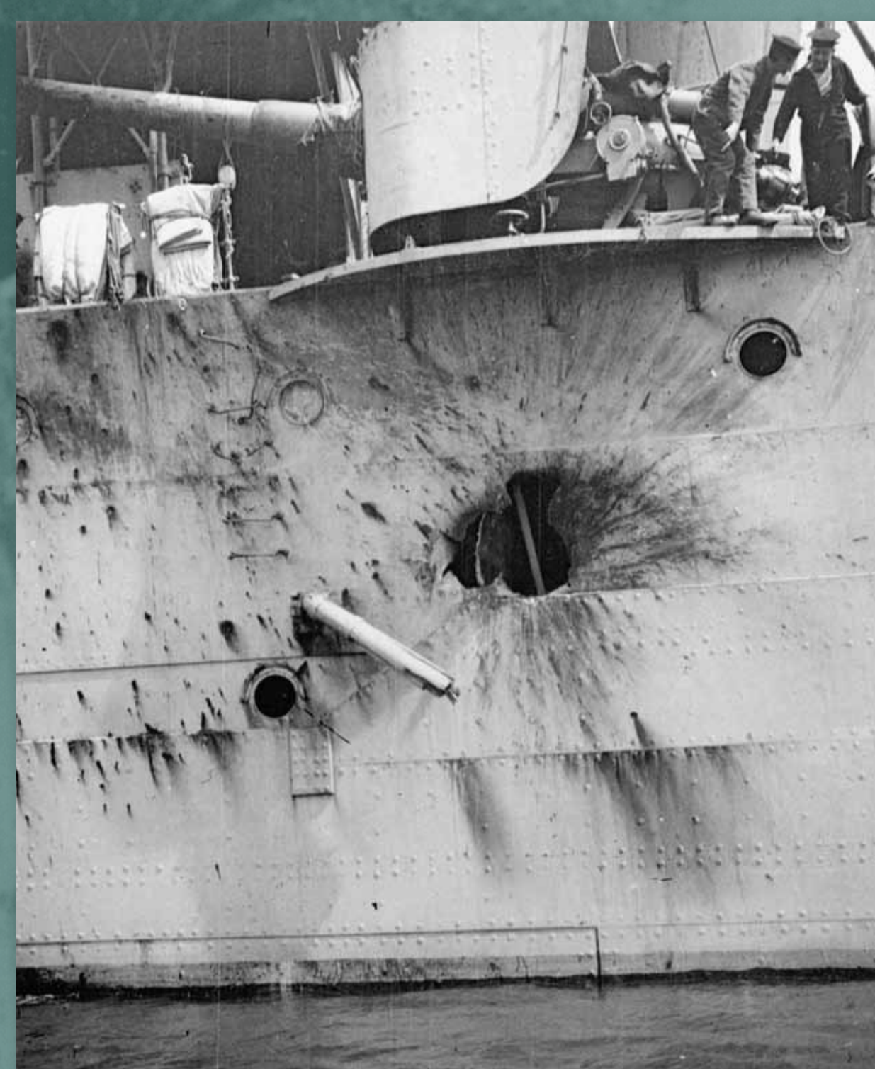
Sailors point to a shell-hole in the side of HMS Chester after the Battle of Jutland, 31 May 1916. Photo courtesy of the Imperial War Museum.
